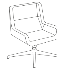
HULOB4S Hush Low Chair 4 Star Base with Standard Glides mm W720 D760 H880 Seat 430 inch W28.5 D30 H34.5 Seat 17
